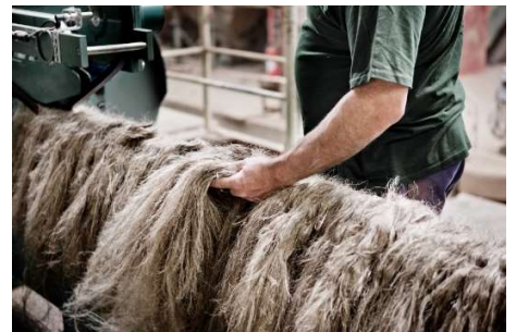
Hemp fibers extracted using a scutcher
